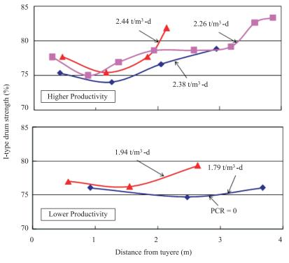
Fig.3. I-type drum strength of coke (%) versus sampling distance from tuyere(m) at various HM productivities.
