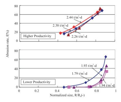
**Fig.6.** Coke abrasion rate (%) versus normalized coke size  $(R/R_0)(-)$  at various HM productivities.
