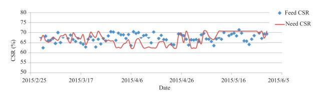
Fig.10. Comparison of daily CSR for feed coke in No. 3 BF and calculated CSR in this study during 2015/3-2015/5.
