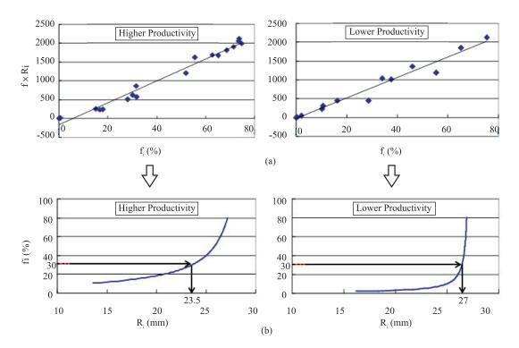
**Fig.7.** (a) [coke abrasion rate  $(f_i) \times \text{coke radius } (R_i)$ ] versus coke abrasion rate  $(f_i)$ . (b) coke abrasion rate  $(f_i)$  versus coke radius  $(R_i)$  from equation (4) and (5).
