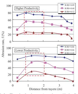
**Fig.9.** The coke abrasion rate (at various residual radius) versus sampling coke distance from tuyere at various productivities.
