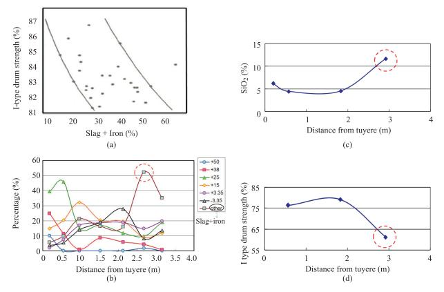
Fig.5. The effects of slag and iron on I-type drum strength of coke.
