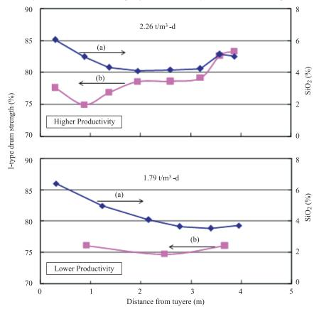
Fig.4. I-type drum strength of coke versus (a)  $SiO_2$  content(%); (b) sampling distance from tuyere(m) at various HM productivities.
